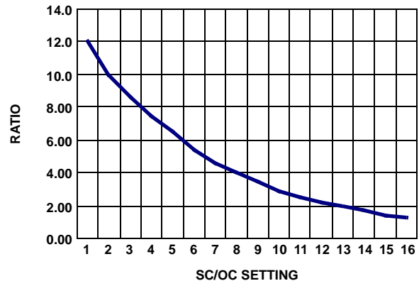
FIGURE 14. SHORT CIRCUIT TO OVERCURRENT RATIO
